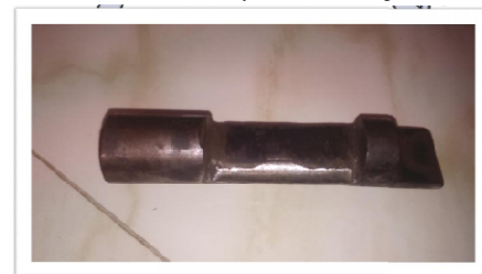
Fig.1.4: Crushing failure of key
